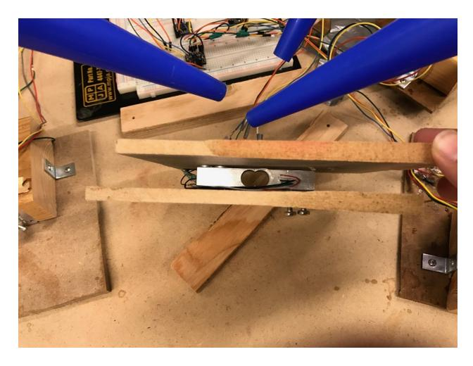
What we have is our 3 pour design surrounding the mixed drink where all four will pour in succession. They are all held up with wooden support on the side through the cups, but attached by a threaded rod specifically cut for it. The actual tilting part of the design is made up of a stand, and lengthwise wooden piece made for certain drink sizes. It is also fitted with seatbelts made of velcro in order to make it so that the drink doesn't fall out when we pour it.
