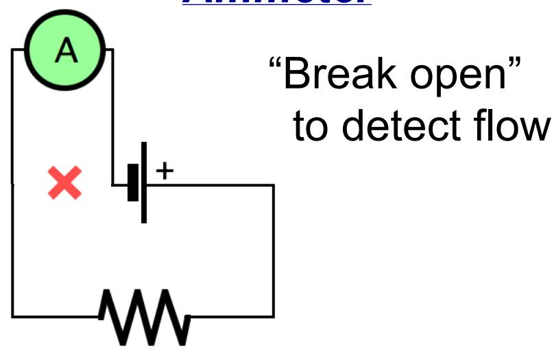
Warning: NEVER connect the Ammeter directly to a battery WITHOUT a resistor!
