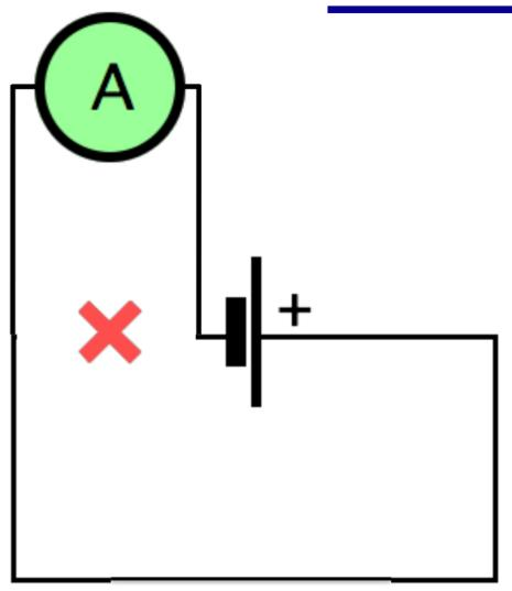
Warning: NEVER connect the Ammeter directly to a battery WITHOUT a resistor!
